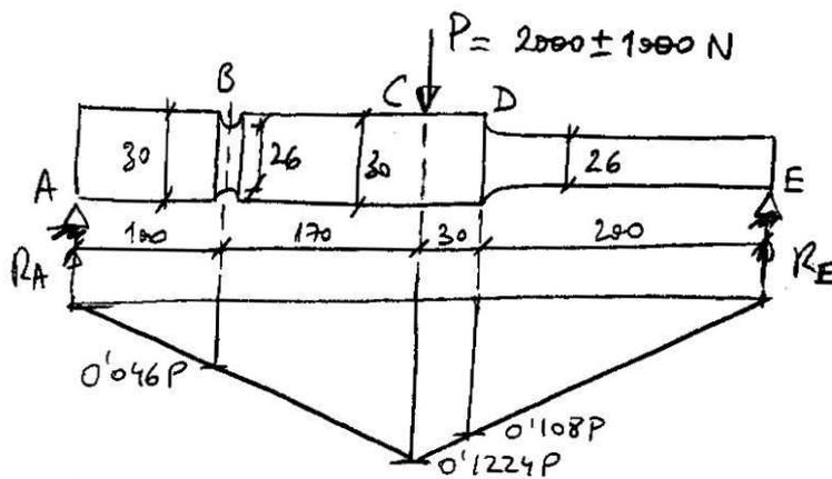
$$\left. \begin{aligned} R_A + R_E &= P \\ R_A \times 500 &= P \times 230 \end{aligned} \right\} R_A = 0.46P \Rightarrow R_E = 0.54P$$
