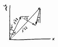
$$\begin{cases} 1^{1}22 \text{ dend} = 0^{1} + 8 \text{ sen } \delta + \alpha_{G/F} \text{ Cos } \gamma + \alpha_{G/H} \text{ den } E \\ 1^{1}22 \text{ cos } \alpha = 0^{1} + 3 \text{ cos } \delta + \alpha_{G/F} \text{ len } \gamma + \alpha_{G/H} \text{ cos } E \end{cases}$$
