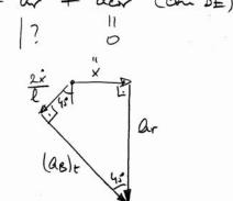
$$\frac{\sqrt{2}(\Omega_{8})_{t} = \ddot{x} + \frac{2\dot{x}}{l} \cdot \frac{\sqrt{2}}{2}}{(\Omega_{6})_{t} = \sqrt{2}\ddot{x} + \frac{2\dot{x}^{2}}{l} = \alpha_{A8}l \implies \boxed{\alpha_{A8} = \frac{\sqrt{2}\ddot{x}}{l} + \frac{2\dot{x}^{2}}{l^{2}}}$$
