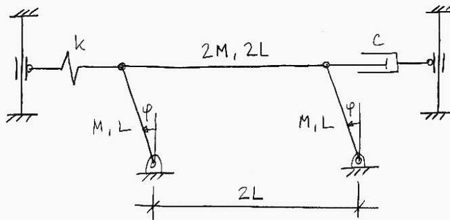
$$T = 2 \times \left[ \frac{1}{2} \left( \frac{1}{3} M L^2 \right) \dot{\varphi}^2 \right] + \frac{1}{2} 2M (L\dot{\varphi})^2 = \frac{4}{3} M L^2 \dot{\varphi}^2$$
