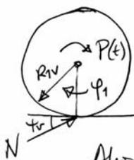
$$P(t) - N R_{1v} \cos \psi_v = I_1 \ddot{\varphi}_1, \text{ luego,}$$
