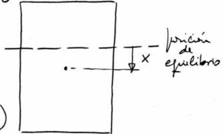
$$x(t) = e^{-\zeta\omega t} \left( x_0 \cos \omega_D t + \frac{\dot{x}_0 + \zeta\omega x_0}{\omega_D} \sin \omega_D t \right)$$
