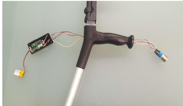
Button in the handle, it has incorporated some LEDs for a visual check of the status of the orthosis
