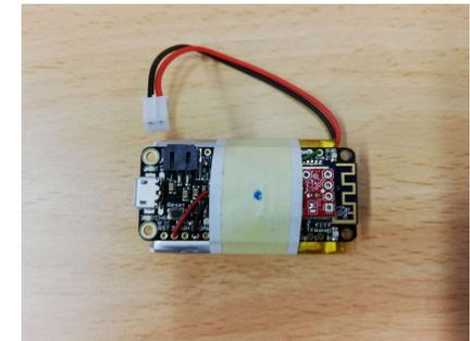
Three sensors are placed along the spine of the user and send data (quaternion of the rotation) at the PC, where is running a Qt application.
