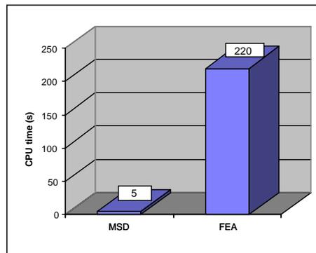
Figure 5. Efficiency of MSD and FEA methods.
