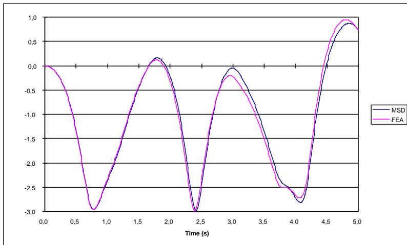
Figure 7. History of the vertical coordinate of the end of a double-pendulum with MSD and FEA methods.
