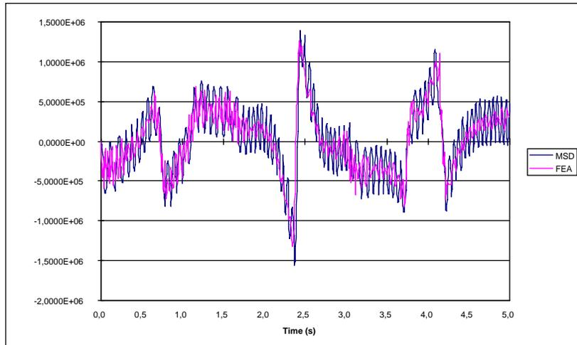
Figure 8. Maximum normal stress at the middle section of the first link of a double-pendulum.
