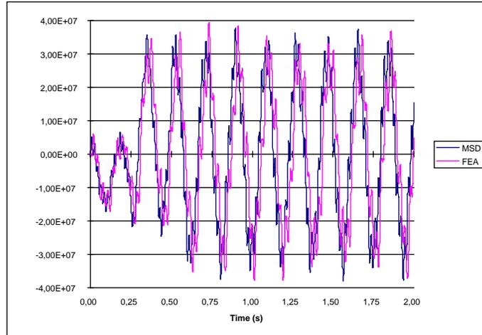
Figure 4. History of the maximum normal stress at the middle section of the beam with MSD and FEA methods.
