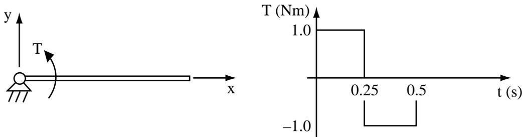
Figure 1. (a) Pinned-free beam. (b) Bang-bang torque.
