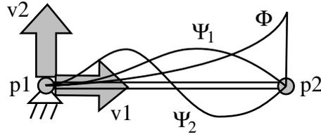
Figure 2. Modeling of a flexible pinned-free beam with the MSD method.
