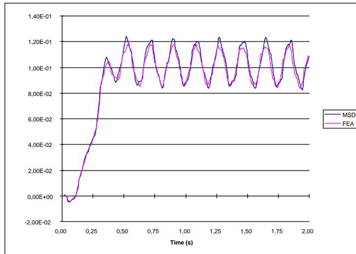
Figure 3. History of the vertical coordinate of the beam with MSD and FEA methods.
