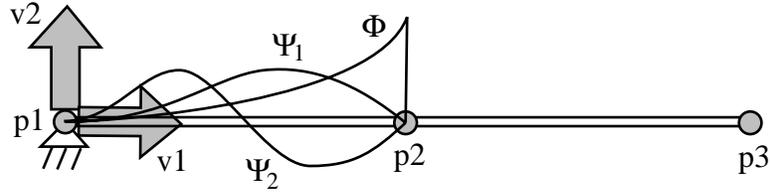
Figure 6. Modeling of a double pendulum with the MSD method.
