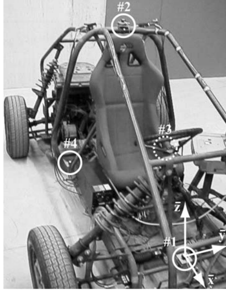
Figure 2: Local reference frame of the chassis and accelerometers situation.
