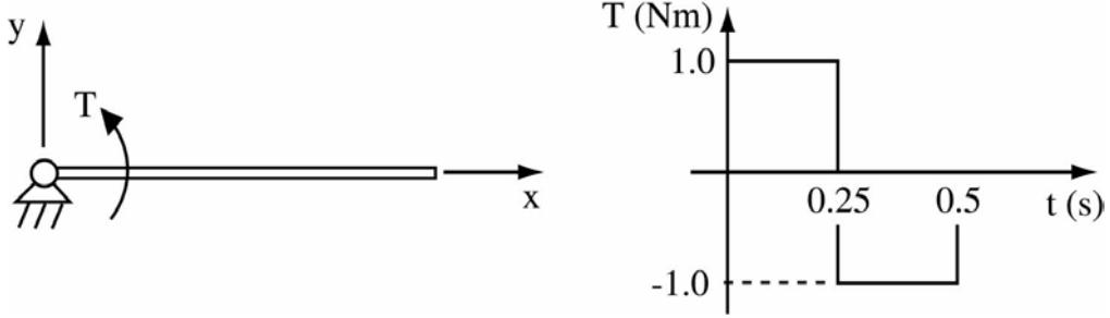
**Fig. 1 a) pinned-free beam; b) bang-bang torque.**
