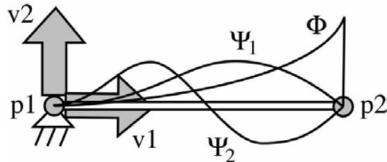
**Fig. 2 Modelling of the flexible pinned-free beam with the authors' method.**
