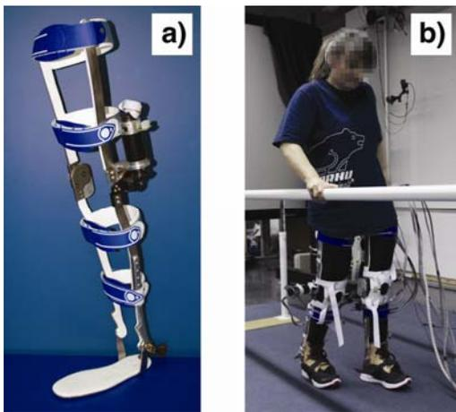
Fig. 2. (a) Prototype with femur-aligned motor. (b) Experimental test of a SCI subject wearing the active KAFO.
