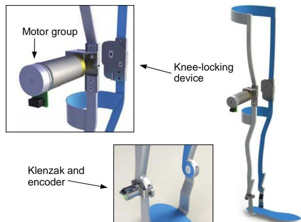
Fig. 1. CAD design of the first prototype of active KAFO.
