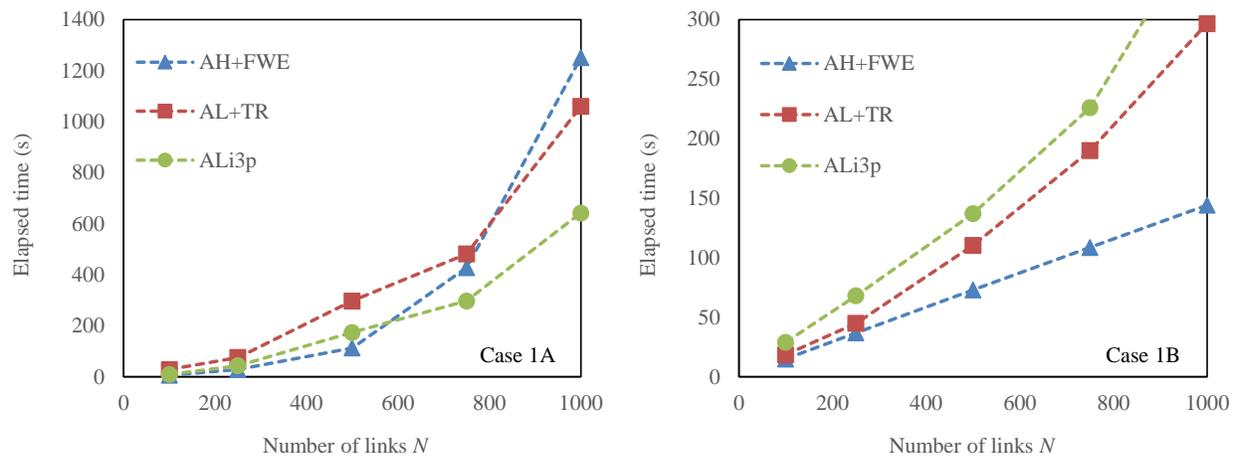
Fig. 2: Effect of the number of links  $N$  on the time required by the simulation of cases 1A and 1B with the three tested algorithms
