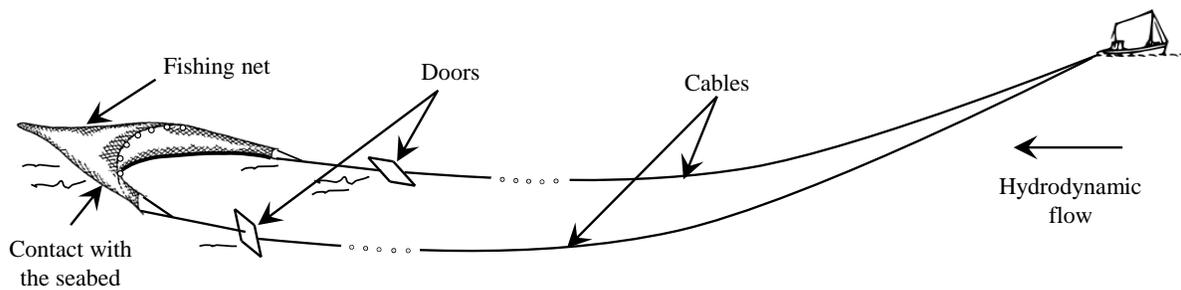
Fig. 1: Components of a fishing trawl net
