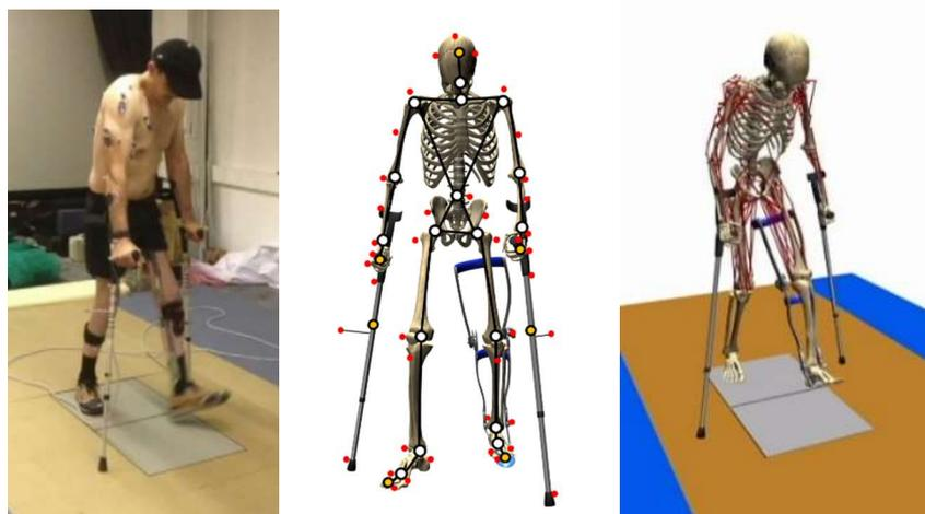
Fig. 1: Gait of SCI subject assisted by passive orthoses and crutches: a) motion-force-EMG capture; b) skeletal model; c) musculoskeletal model.
