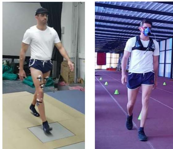
Fig. 3: Energy consumption in a healthy subject: a) motion-force-EMG capture; b) 5-minute test with portable gas analyzer.
