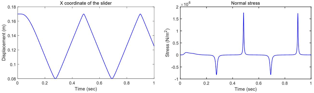
Figure 1: Displacement of the X coordinate of a point of the slider (on the left) and normal stress at the center of the middle section of the rod (on the right).
