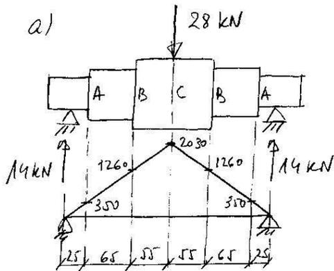
$$\begin{cases} M_C = 14000 \times 0.145 = 2030 \text{ Nm} \\ M_B = 14000 \times 0.09 = 1260 \text{ Nm} \\ M_A = 14000 \times 0.025 = 350 \text{ Nm} \end{cases}$$
