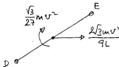
$$I_{BC} = \frac{1}{12} m (2L)^2 = \frac{1}{3} mL^2 ; \quad I_{BC} \alpha_{BC} = \frac{1}{3} mL^2 \frac{\sqrt{3}v^2}{9L^2} = \frac{\sqrt{3}}{27} mv^2$$
