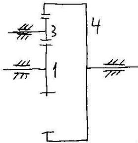
$$\frac{\bar{\omega}_4}{\bar{\omega}_1} = -\frac{z_1}{z_4} \Rightarrow \frac{\omega_4 - \omega_2}{\omega_1 - \omega_2} = -\frac{60}{120}$$
